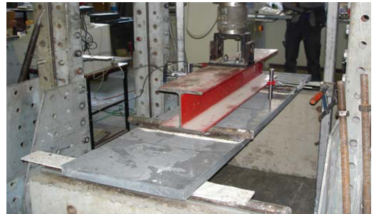
Figure 3. Four-point bending test for UHPC cladding panels.
