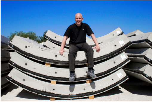
Figure 11. Steel-fibre reinforced concrete segments of the Copenhagen Heating Tunnel.
