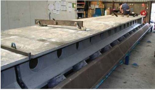
Figure 13. Demoulding of match-cast segments.
