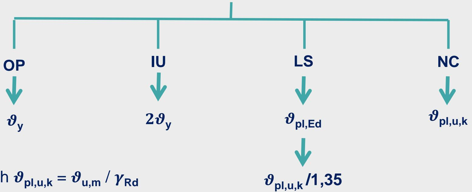
The **mean value** of plastic contribution of ultimate chord rotation may be derived by a physical model, which assumes that the plastic part of curvature is uniform within the **length of plastic hinge** ( $L_{pl}$ )
