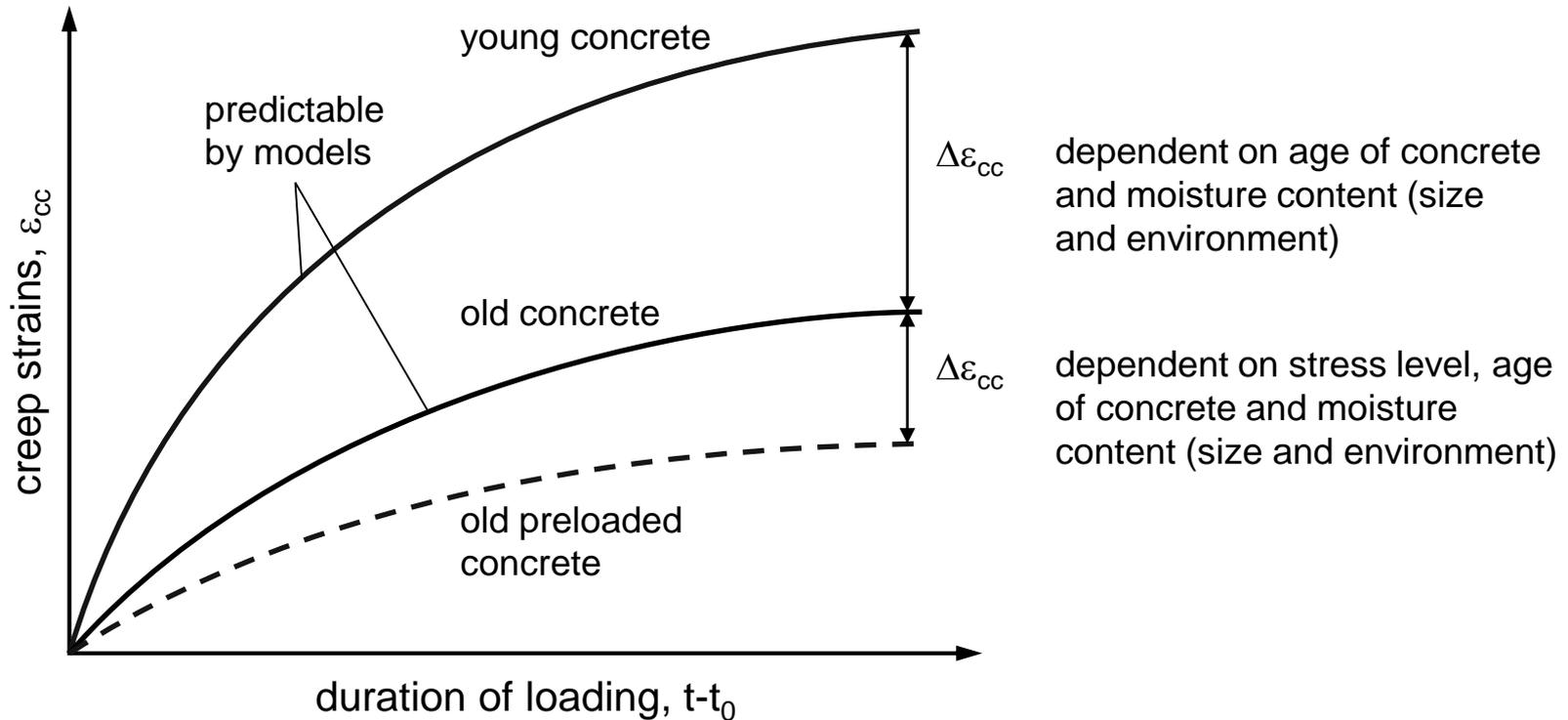
For creep sensitive old structures tests are required.
