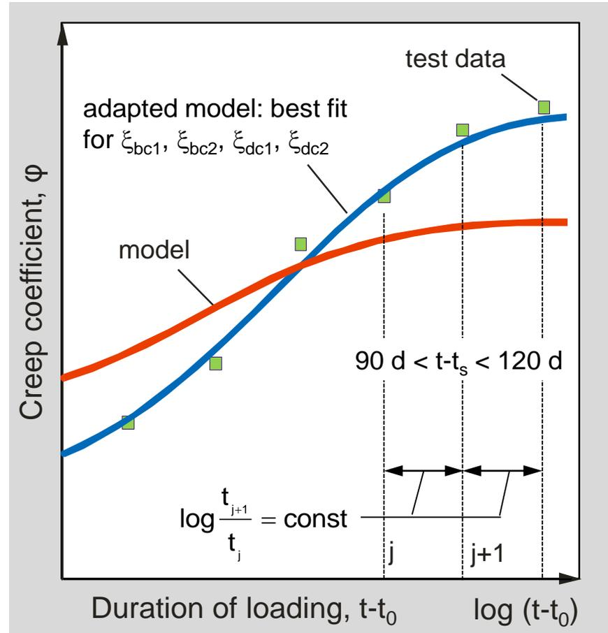
**Accuracy gain through tests: Coefficient of variation drops from  $V \approx 30\%$  to  $V \approx 10\%$**
