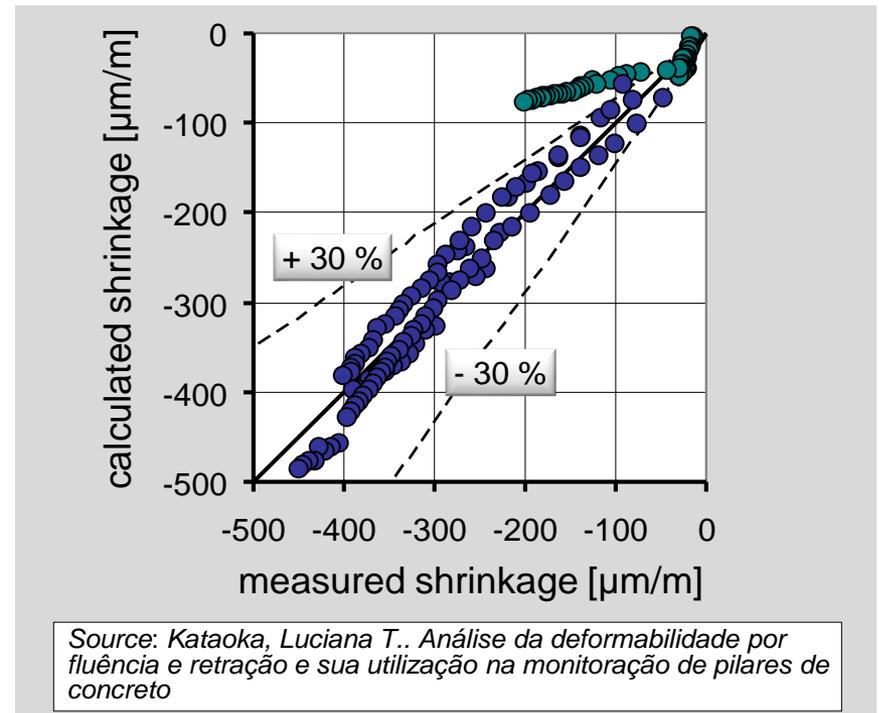
The model predicts the total shrinkage deformations for NSC and HSC very well. For HSC a poor prediction of basic shrinkage was seen. However, this is just one test!
