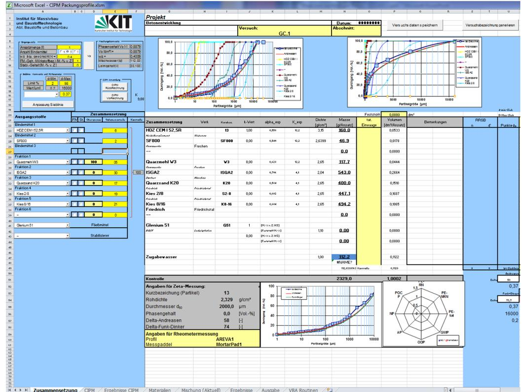
Excel based software calculates optimal packing density based on the models of Andreasen, de Larrard, Fennis and own works
